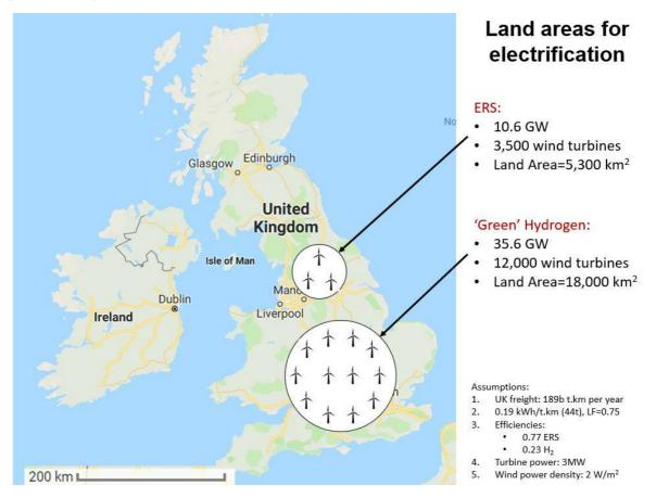
Estimated land areas of wind turbines needed for powering the UK's heavy goods vehicles by electric road system or via 'Green' Hydrogen (electrolysis)
